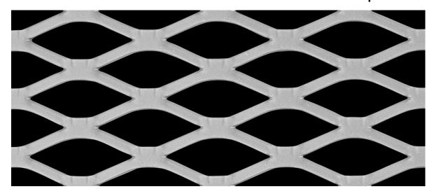
LW Aperture:42.93mm (50.80mm Pitch)Strand Width:4.60mmSW Pitch:14.22mm (23.42mm Pitch)Thickness:2.69mmWeight:8.59 kg / m2 (Black Weight)Open Area:61%
